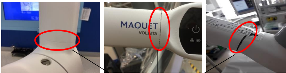
Pictures of the coating crack with different size
