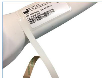
Place the adhesive strip covering the coating crack
