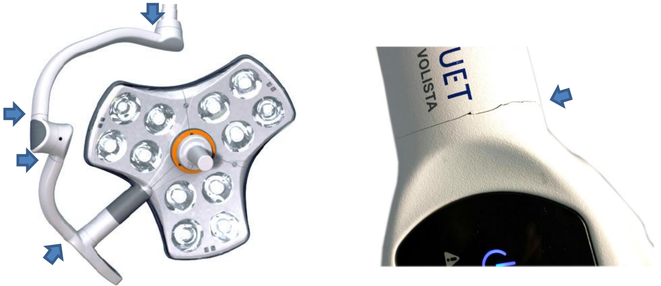
Fig. 1: Coating crack phenomenon
