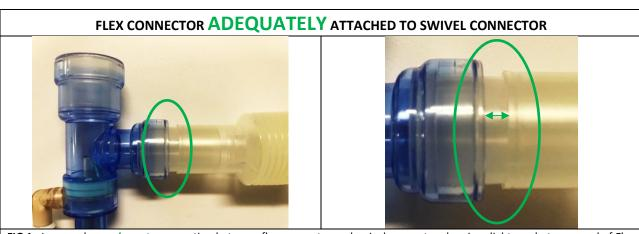
**FIG 1.** Images show *adequate* connection between flex connector and swivel connector showing slight gap between end of Flex Connector and adapter. (Please note the closed suction adapter is available in blue or white/clear.)
