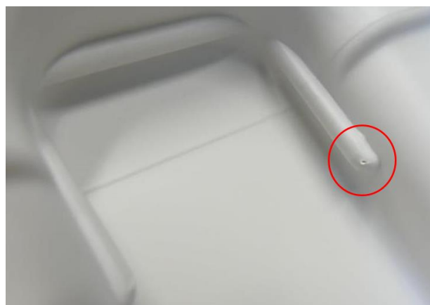
Example for a crack in intellipack packaging tray
