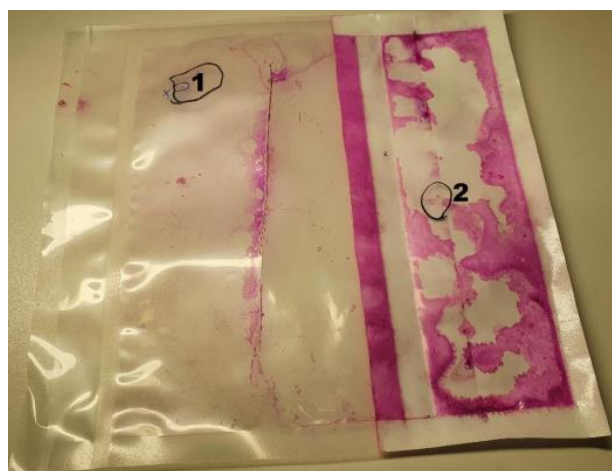
Example for a crack in intellipack packaging tray
