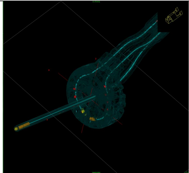
Figure 6: Incorrect (mirrored) 3D view when using the Triangles option for Applicator skin visualization.
